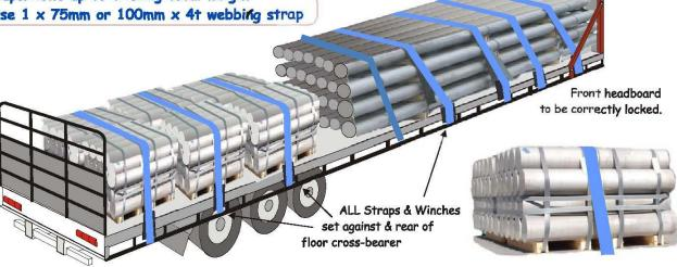
Total lashing may appear to be excessive, against LRG tables but additional pretension & LC is recommended for both long & short billets.
