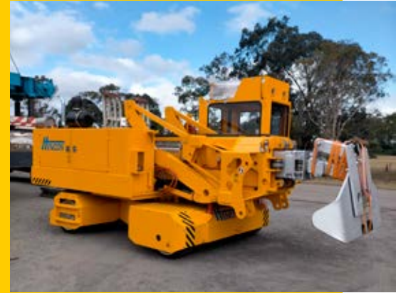
One of TAC's new Casthouse Furnace Tending vehicles
